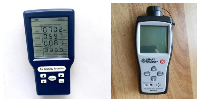
Figure.2 air quality tester and ammonia smart sensor
