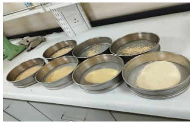
Figure (3): photo during separation on different sieve sizes of the flour sample
