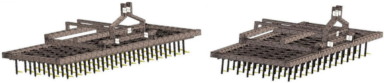
Figure (5): The mesh of nodes and finite elements for the (circular and rectangular) spike tooth harrow.
