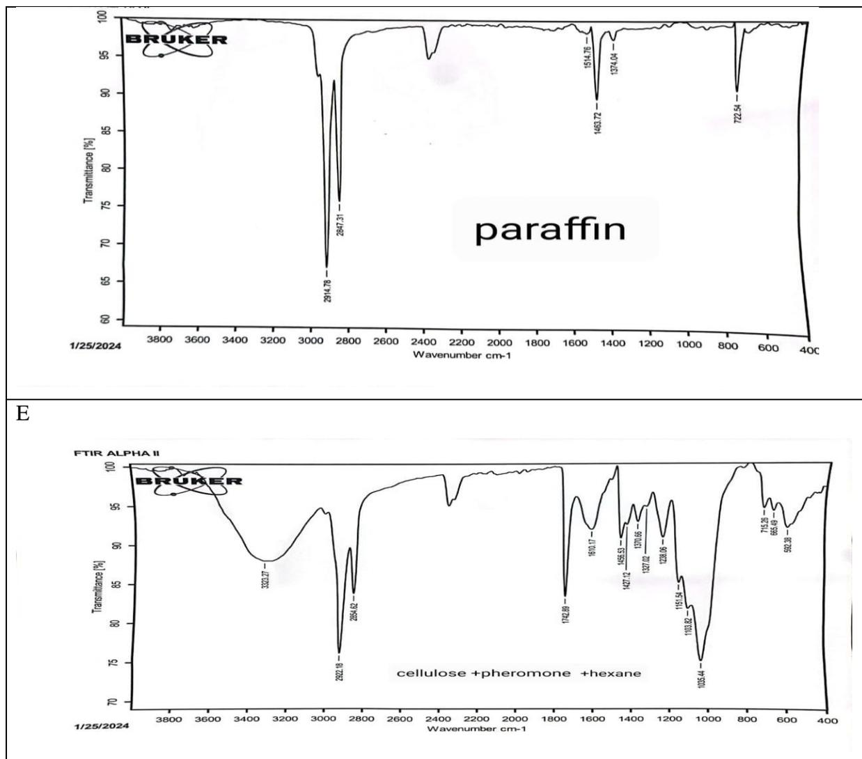
**Figure 6:** A: FTIR analysis of cellulose fibers (cellulose) B: FTIR analysis of the mixture of holocellulose and pheromone extract with n-hexane C: FTIR analysis of n-hexane D: FTIR analysis of paraffin E: FTIR analysis of the mixture of paraffin and pheromone extract with n-hexane.
